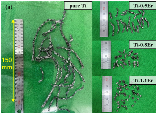
Fig. 8. Pictures showing the drilling machine used in this study and Ti chips produced during the drilling test: (a) pure Ti sample, (b) Er-added Ti sample (1.1 wt.%). The cutting chips of the Er-added Ti sample do not stick to the cutting tool while those of the pure Ti sample do (yellow circle).
