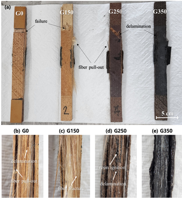
Fig. 5. (a) Failure modes of specimens: G0, G150, G250, and G350. Cross-sectional failure modes of specimens: (b) G0, (c) G150, (d) G250, and (e) G350.
