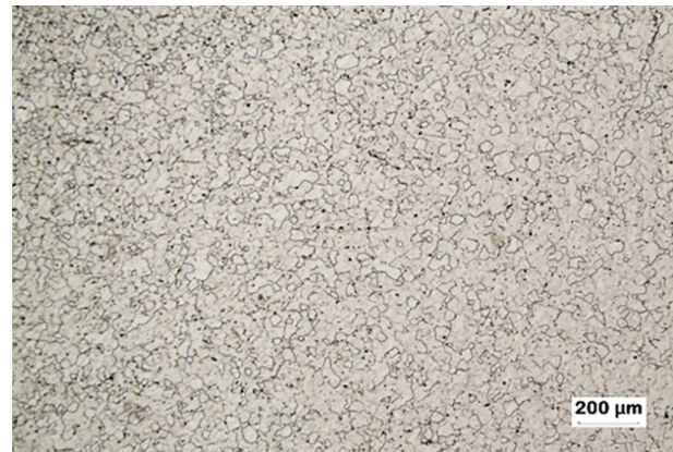
Fig. 2. Optical micrograph of the as-received Ti-12.1Mo-1.0Fe alloy.
