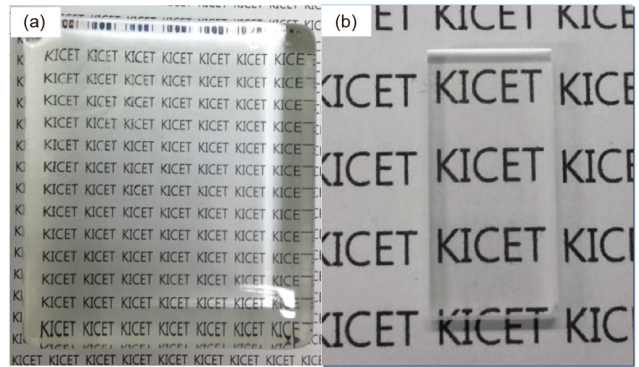
Fig. 2. Photographs of bulk samples: (a) before polishing and (b) after polishing.
